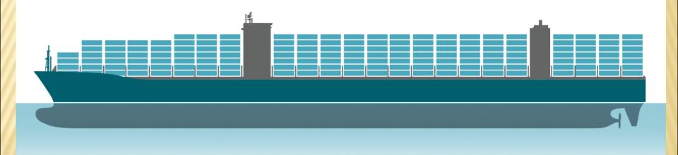
Length: **400m** Speed: **22.8 knots**  Built: **2018** Gross tonnage: **219,076**
